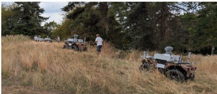
(a) A composite image showing the Barakuda UGV during data collection via manual teleoperation.
