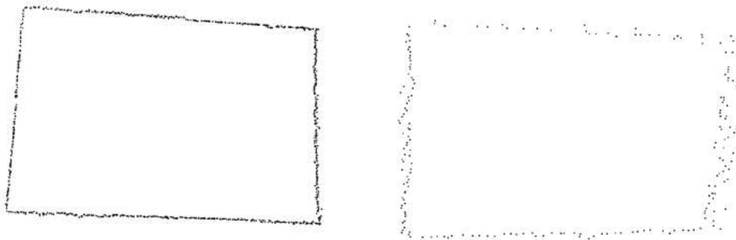
Figure 5: Two extracted mirror contour as 3D point clouds of mirrors. The right side features always more noise, since the incidence angle is much smaller there.
