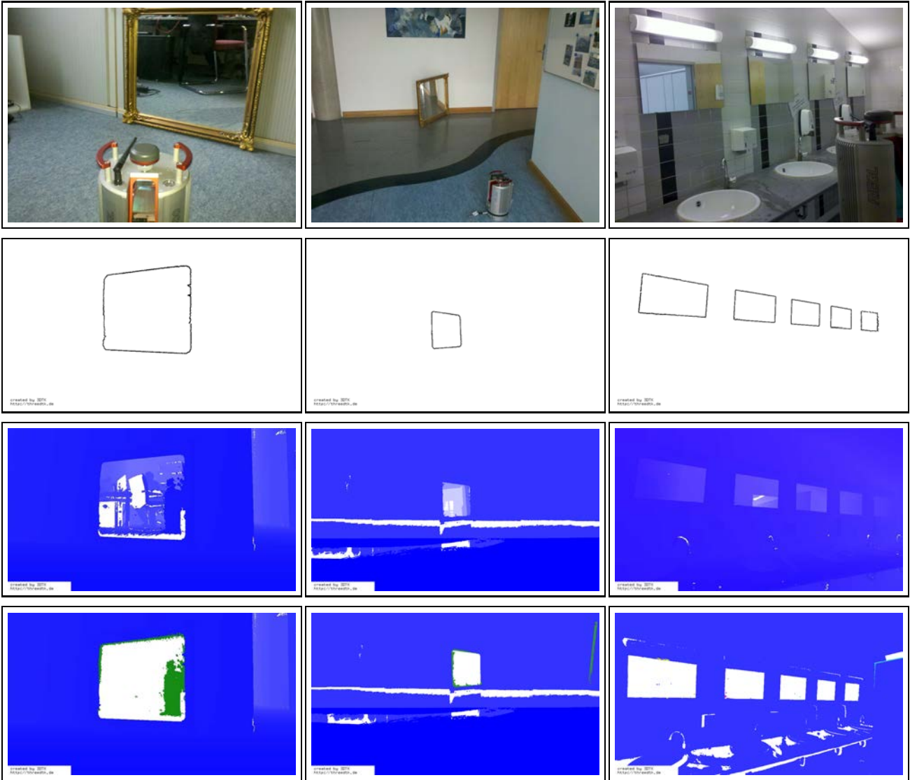
Figure 4: Left: Mirror of size 56 \times 64 cm in an office environment. Middle: Same mirror placed in an office corridor. Right: 5 mirrors of size 40 \times 60 cm in a bath room. Top row: Photo of the scenes. Second row: Extracted 3D contours. Third row: Screenshots in a 3D point cloud viewer without mirror correction. Bottom: Corrected 3D point clouds.
