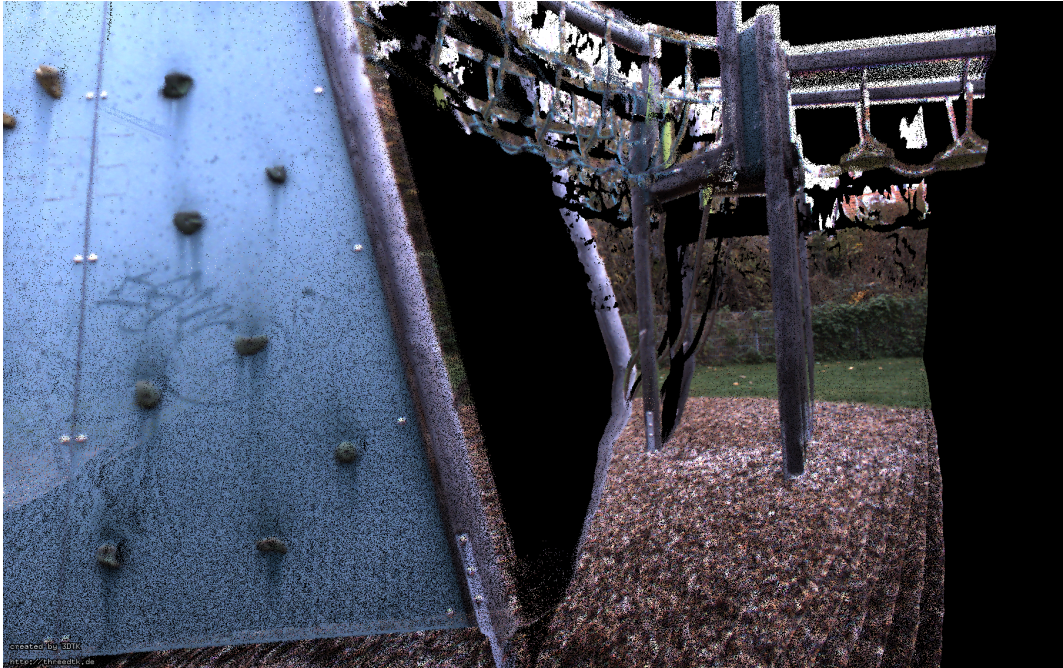
Figure 3.16: Big deviation at the right edge of the climbing wall
