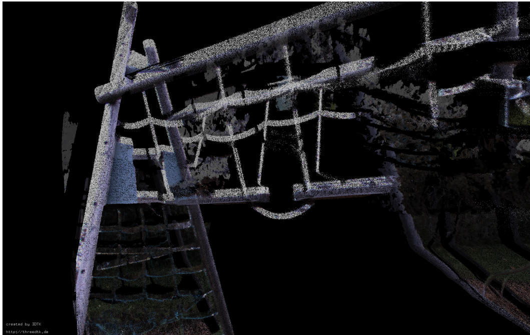
Figure 3.18: Big deviation in y at the hanging bars.
