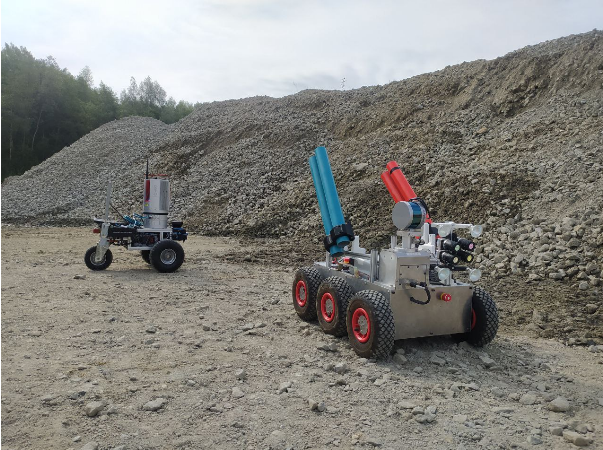
Figure 3.2: The robots that the astronauts will control: Robot “Lars” (left) with a laser scanner and “Charlie” (right) with four monochrome cameras for rock analysis and the sensor distribution system to launch UWB sensors.
