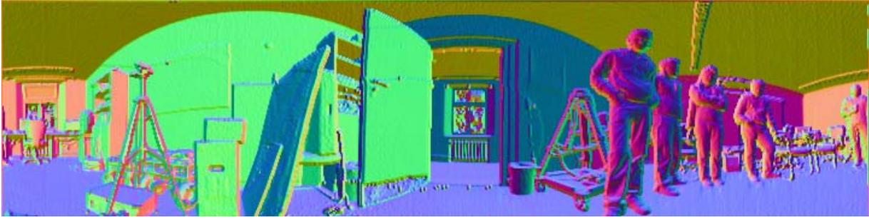
**Figure 5.7:** The normal vectors computed from the point cloud from Figure 1.1 using the optimized LS method.
