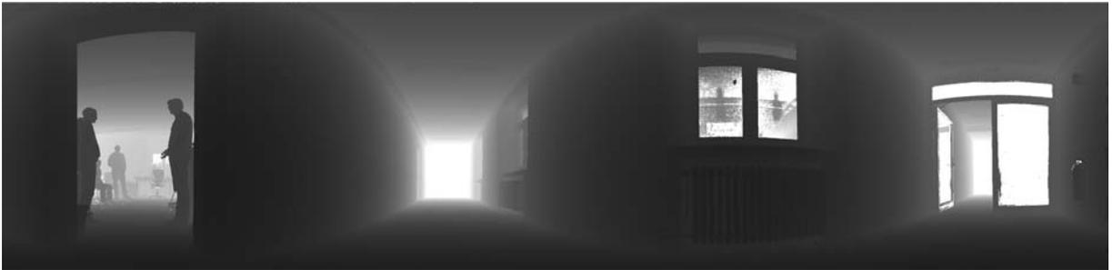
**Figure 1.2:** An example SRI image. The 360 degree view allows to present the whole point cloud. The elevation range here is 100 degrees but can also be adjusted to show the whole span of the cloud or just a desired part. Note that in this image only ranges upto 10 m are shown in order for the image to be perceivable.
