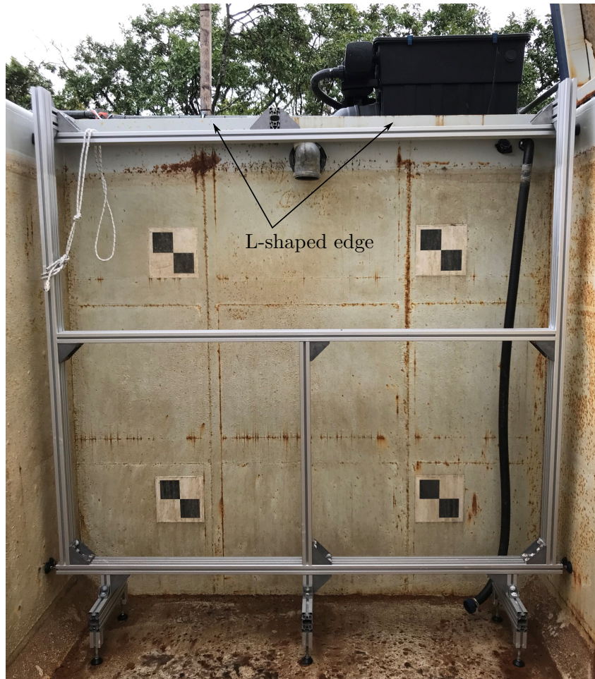
Figure 4.2: Photo of the mounted framework in the container
