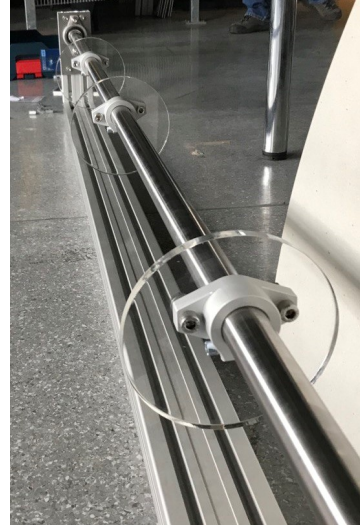
(b) Image of all middle sockets mounted on the metal shaft.
