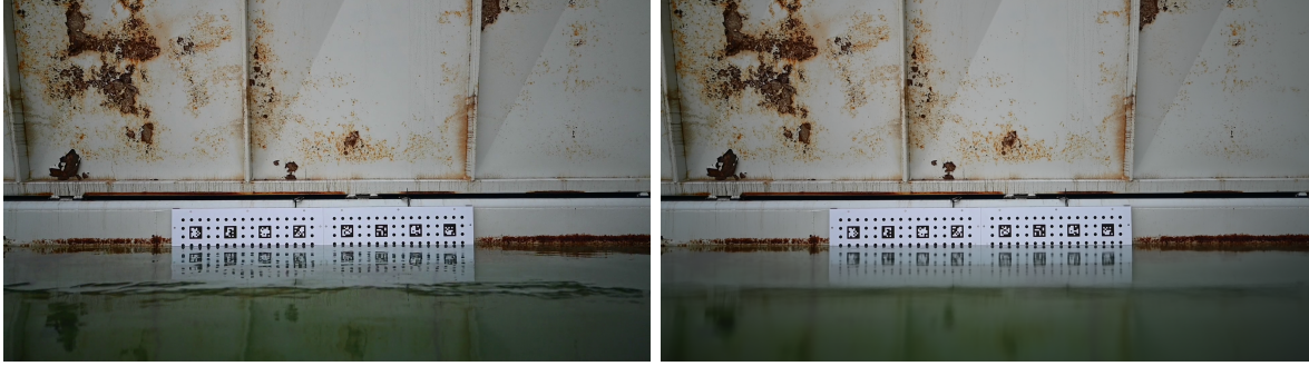
(a) Image extracted from the video of a water surface without produced waves that is used in the Fluidity program [6]. (b) Resulting image with 10 iterations of the Fluidity algorithm [6] with a video of a water surface without produced waves as input
