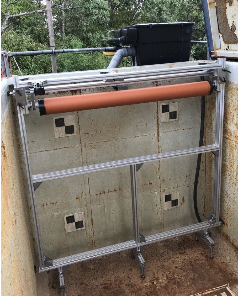
Figure 4.15: Image of the eccentric roller wave generator build in the framework that is mounted in the water container.
