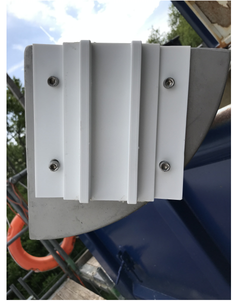
(b) Image of the 3D printed plastic glider screwed on the cylindrical plunger.
