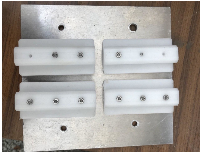
Figure 4.6: Image of the DOLD Mechatronic glider [12] that are screwed on the metal plate. This construction makes the connection between the framework and the cylindrical plunger.
