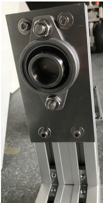
(a) Image of the used ball bearing to fix the metal shaft in the aluminum profile framework.
