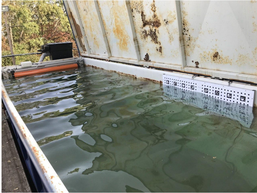
Figure 5.1: Image of the experiment setup with the eccentric roller and the Aruco marker board [7] in the water container.
