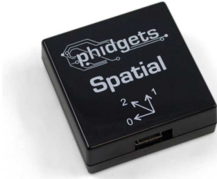
(a) Phidget Spatial 3/3/3 No.1044.1b [31], used for retrieving pose data
