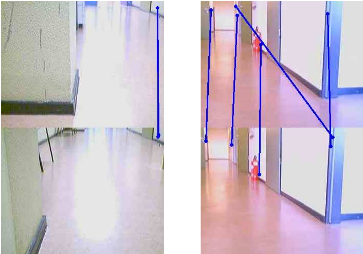
Figure 4.3: The left picture shows an example for a false positive. Although the scenes looks similar, the images show two different locations. On the right picture a true positive is shown, but one feature descriptor was matched incorrectly.
