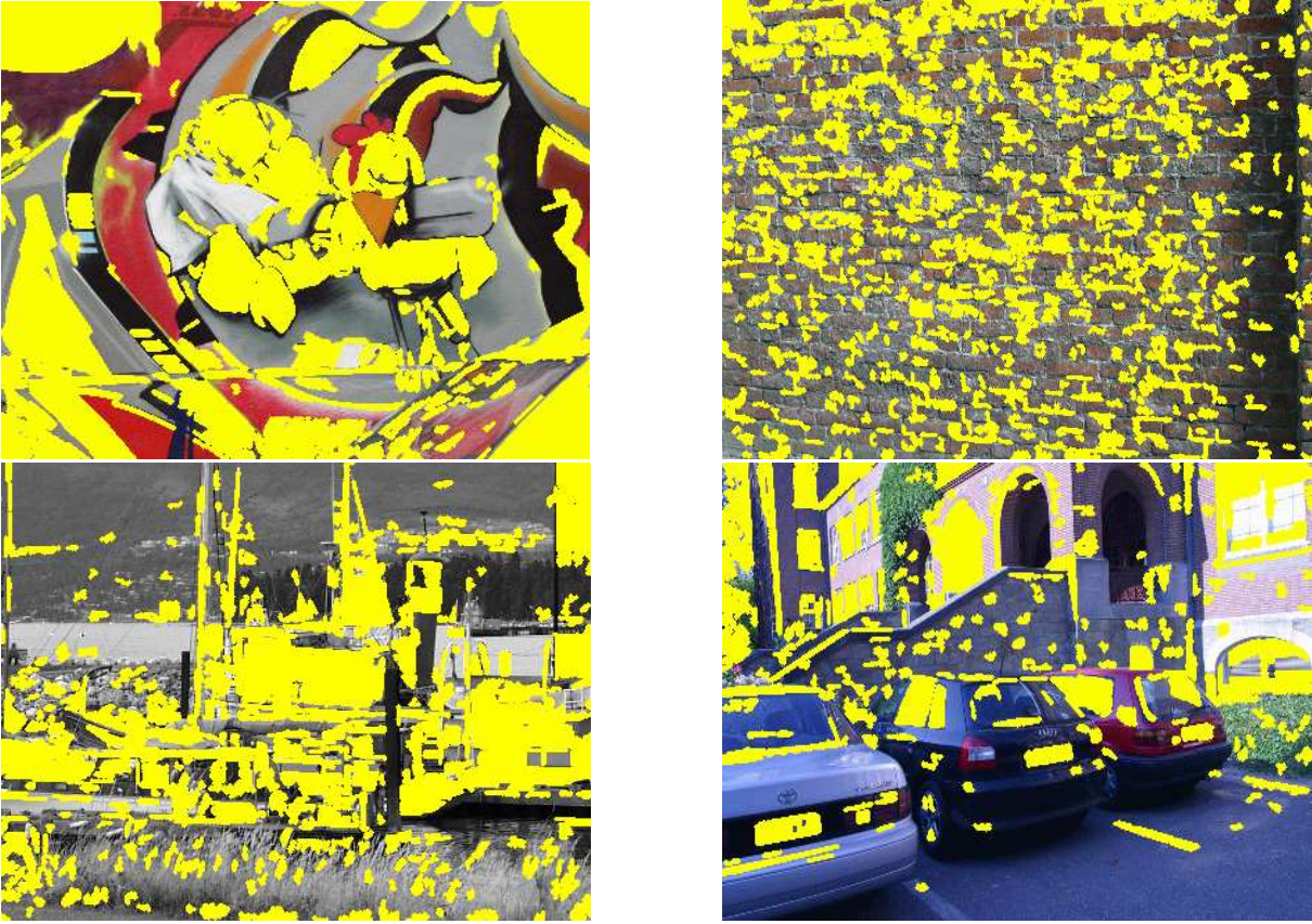
Figure 2.5: MSERs in various scenes. The images are from the data set that is illustrated in Figure 3.1. In contrast to the salient regions, which are shown in Figure 2.3, the shape of a MSER is arbitrary.
