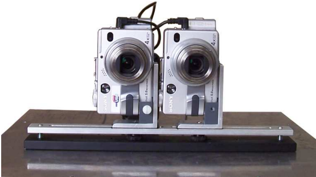
Figure 2.1.: Stereo Rig with two digital cameras mounted. The black cables on the top are connected to the synchronization device.
