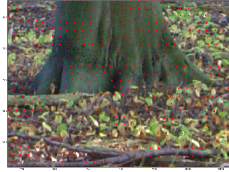
Figure 3.2.: Laser Scanner data projected onto one image pane
