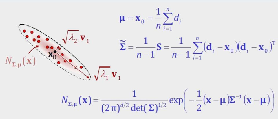
PCA can be interpreted as fitting a Gaussian distribution and computing the main axes
