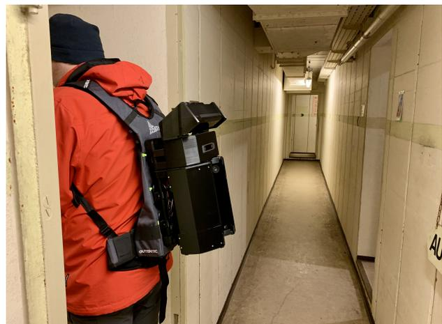
Figure 1. Proposed indoor mapping backpack with four Microsoft Kinect 2 RGB-D cameras and an Intel T265 stereo camera for visual-inertial odometry.
