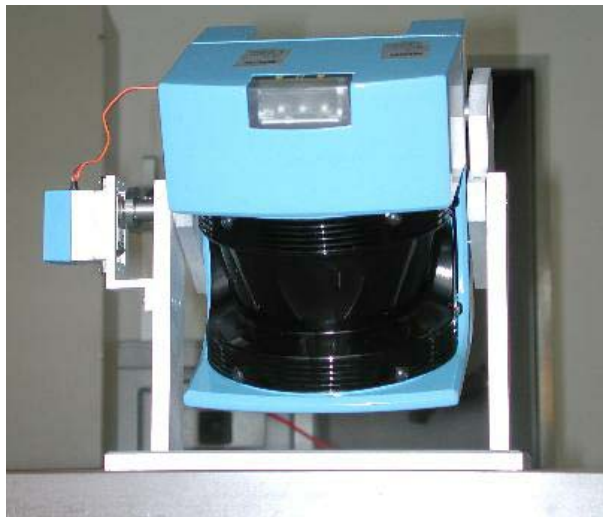
Fig. 4. The AIS 3D laser scanner, as based on a SICK LMS [1].
