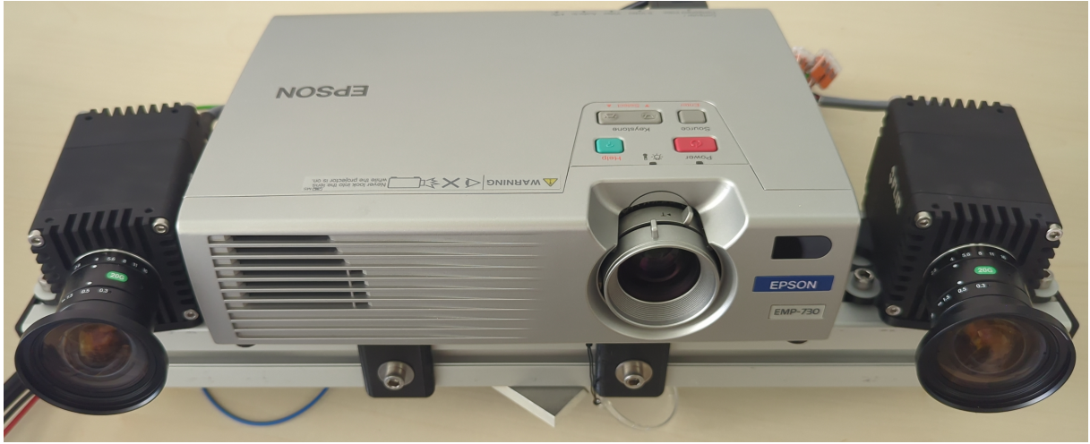
Figure 4.1: The stereo scanning setup.
