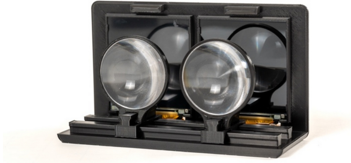
Figure 4.3: First headset prototype with movable lenses directly in front of the displays.
