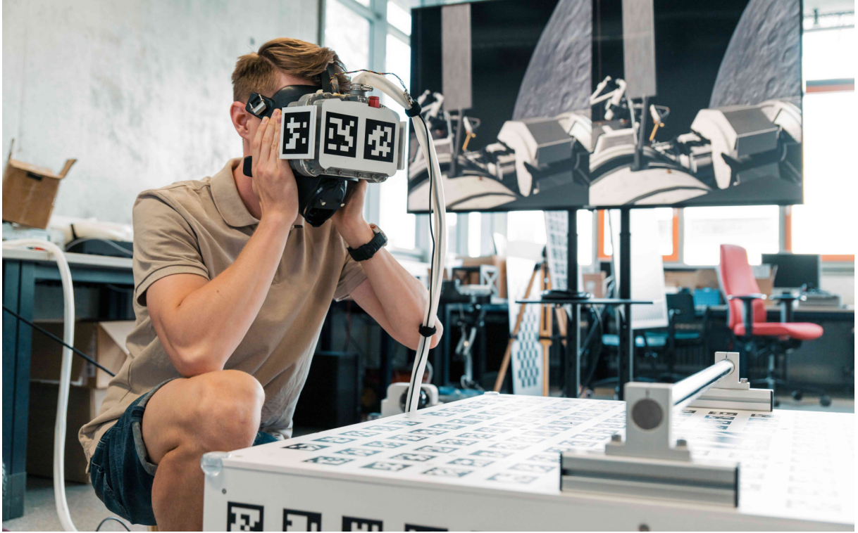
Figure 4.4: Trying out the headset mounted on diving mask with AprilTag fiducial markers attached to sides. The virtual environment rendered on the headset’s displays is mirrored to a monitor in the background.
