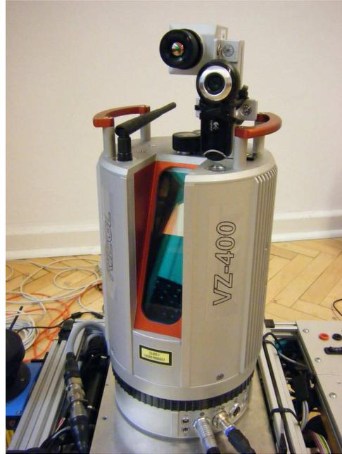
**Figure 1.1:** A sensor system consisting a video camera and thermal camera mounted on of a laser scanner. (Source: [5])
