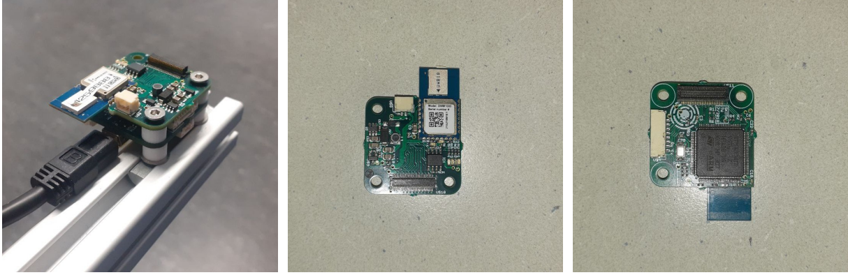
(a) UWB PCB mounted in a stack with a USB communication board on the robot.
