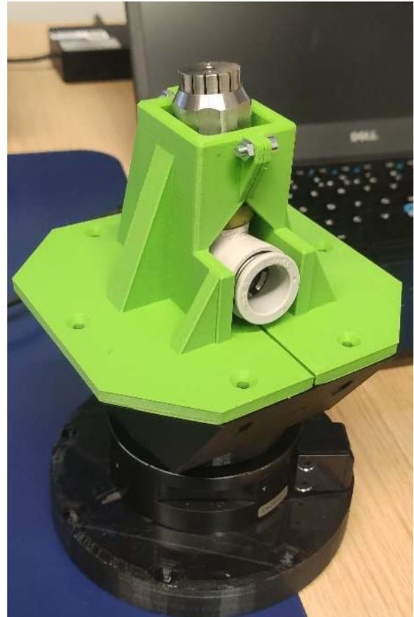
**Figure 3.3:** Thruster test stand. Technical drawing (left) and 3D-Printed stand (right) using the ATI Gamma Force Torque sensor FT5243 [13]. The force-torque sensor is mounted on the base. On top, an enclosure for the thruster is mounted (in green). The air inlet is routed to the side such that the thruster expels the air to the top and thus pushes down onto the force-torque sensor.
