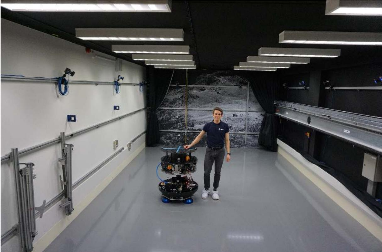
**Figure 1.1:** The author with the testing platform on the flat-floor of the ORGL at ESTEC. A flat ground on which an air-bearing platform can float. The testing platform consists of three subsystems: the floating base ACROBAT, the thruster and tank assembly SATSIM, and the RW REACSA, which are stacked onto each other. The flat-floor is within the field-of-view of a Motion-Capture (MoCap) system that provides pose measurements to some previously defined world reference frame.
