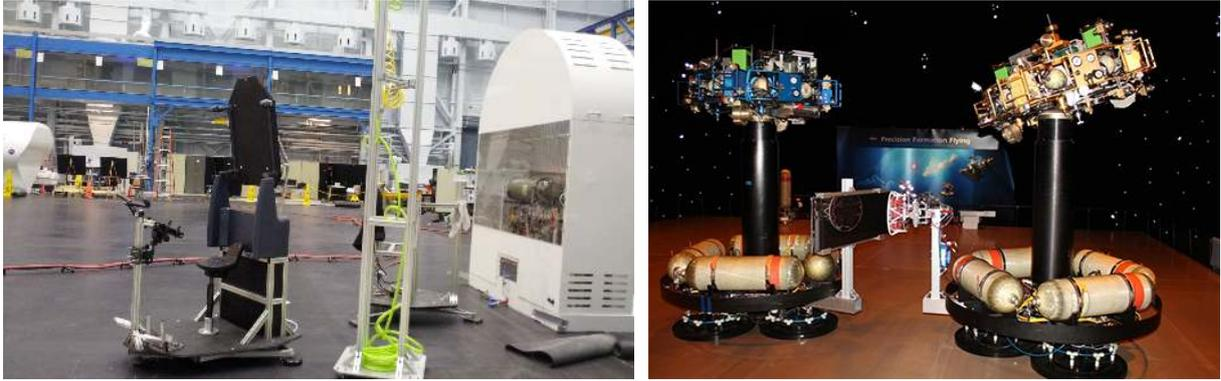
**Figure 2.1:** Left: the Air Bearing Platform at the Johnson Space Center in Houston. Courtesy of NASA. The black area is the epoxy flat-floor. In the front, the image depicts a human-operated hovering platform [1]. Right: The Formation Control Testbed (FCT) at JPL [2].
