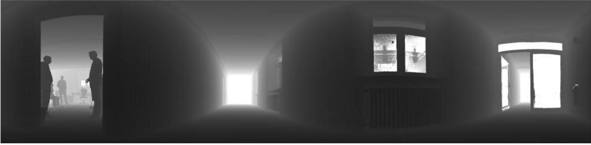
**Figure 4.8:** Spherical range image (SRI) obtained from a 3D point cloud. Source: [41]
