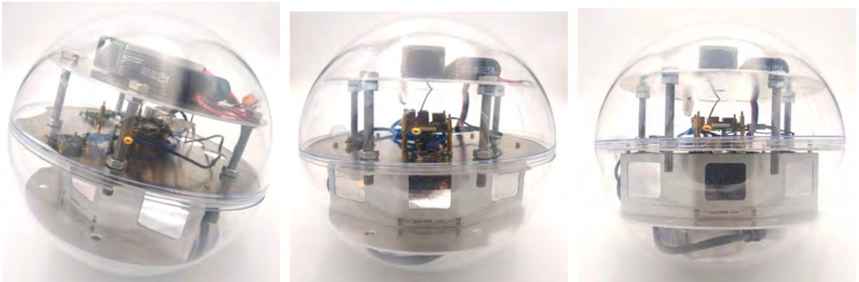
**Figure 5.7:** Prototype used for data acquisition with the rolling sphere. The main payload is the Livox Mid-100 laser scanner. For pose-estimation, three IMUs of the manufacturer Phidget are placed inside and a Raspberry Pi 4 for the calculations. On the top are two batteries, and on the bottom one voltage stabilizer and the breakout box of the laser scanner.
