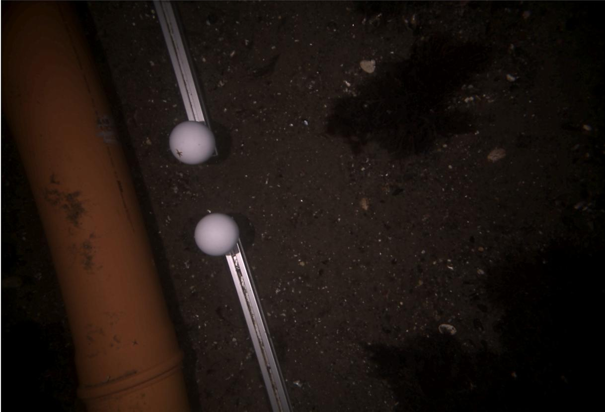
**Figure 7.4:** Snapshot of a data set from the *UWSensor* project during a trajectory under water. The spheres seen here are used in the evaluation of the resulting point cloud.
