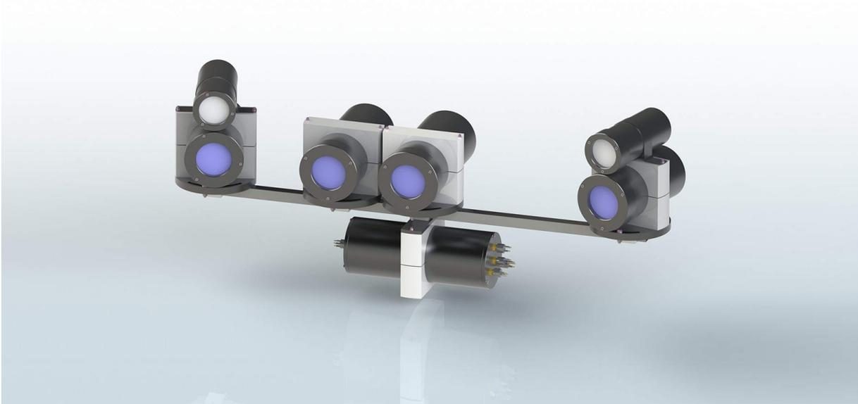
**Figure 1.2:** Preliminary design of the sensor platform of the *UWSensor* project<sup>2</sup>. The two outer housings each contain a 3D measurement camera and an additional light source. In the center housings, an additional color camera is installed, which is used for the visual odometry, as well as the fringe projector and the control unit of the sensors. One IMU is installed in each of the two lower housings, with the second one serving as a redundancy. The device has a width of about 1m.
