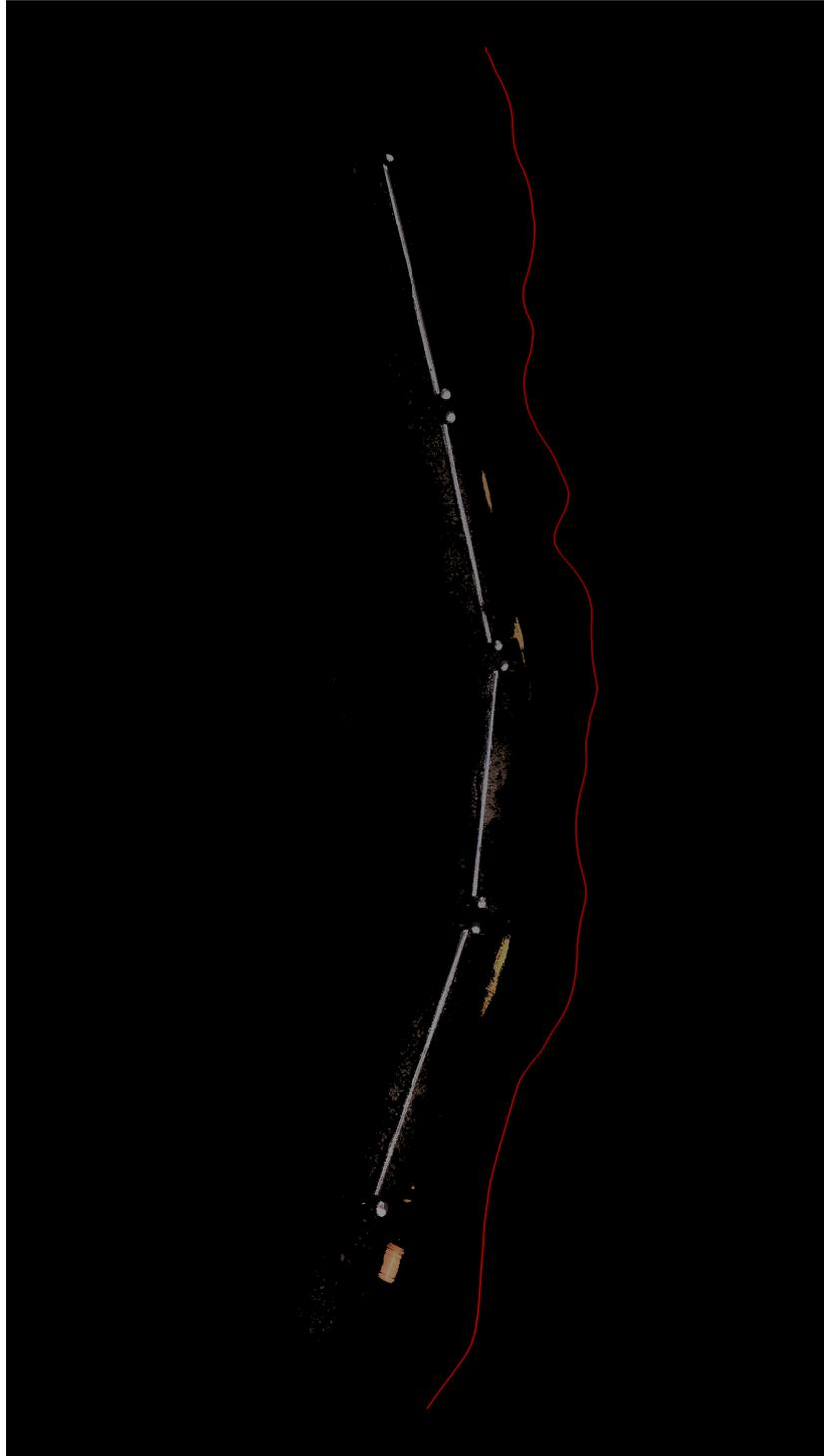
**Figure 7.5:** Point cloud generated by *UWSensor*, which was colored using the color camera data. *VINS-Mono* was used to estimate the poses, using the translation and rotation between the camera and IMU estimated as part of this thesis. The trajectory determined using this is shown as a red line. Areas which can be recognized as circles are the spheres which is seen in Fig. 7.4. The trajectory starts at the top of the figure and ends at the bottom.
