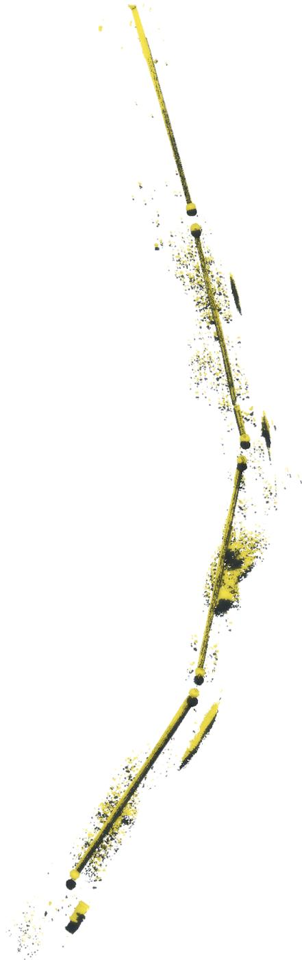
**Figure 7.6:** Shows the point clouds generated by *UWSensor*, which were estimated using the native *VINS-Mono* (black) and the resulting point cloud using the translation and rotation between the camera and IMU estimated as part of this thesis (yellow). Areas which can be recognized as circles are the spheres which is seen in Fig. 7.4. The trajectory starts at the top of the figure and ends at the bottom.
