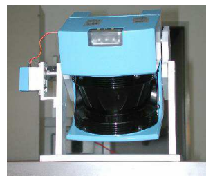
Fig. 1: 3D laser scanner. Its technical basis is a SICK LMS-200.
