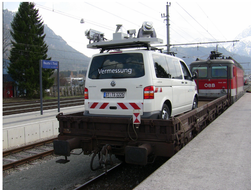
Fig. 11. The Optech Lynx Mobile Mapper on the back of a train wagon.
