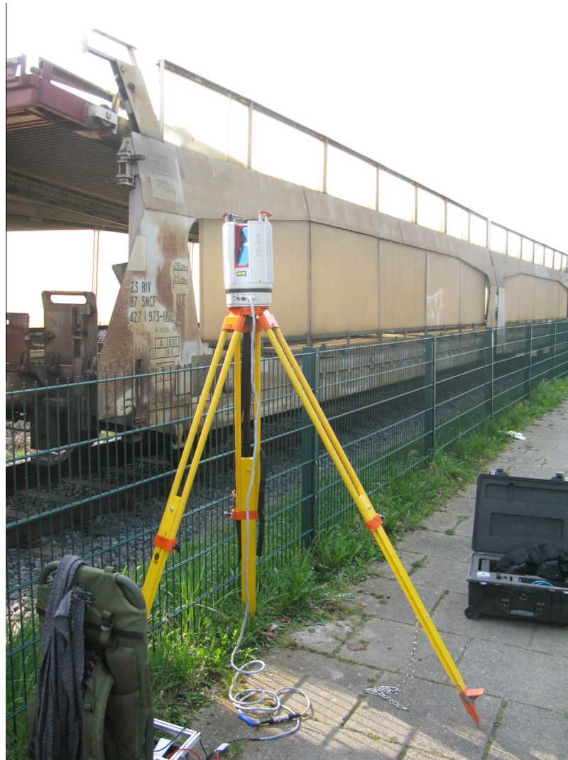
Fig. 13. The Riegl VZ-400 laser scanner set up next to the train wagon.
