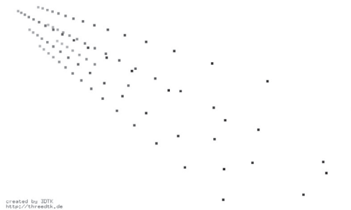
(e) Minimum point distance d_m = 0.924 m for a search radius of r = 0.8 m makes a model with 93 points.
