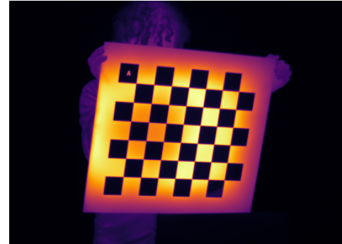
Fig. 3: Custom two-layer FR4 PCB calibration board for thermal camera. Copper and substrate regions provide distinct emissivity contrast when heated, enabling reliable corner detection.
