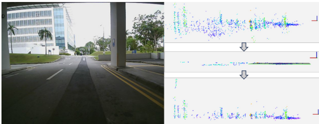
Fig. 3: Ground Extraction. left: camera view, right side from top to down: radar inliers, ground detection and fitting, non-ground filter
