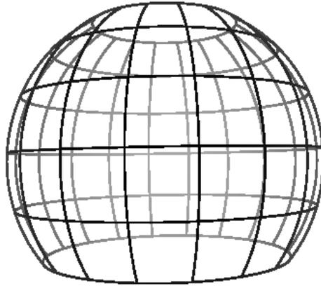
Figure 2: A scanned environment as an artificial sphere with respect to the field of view of the scanner with the scanner positioned at the center of the sphere.
