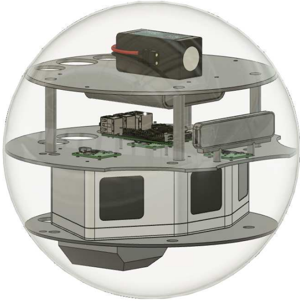
Fig. 3: The spherical robot used for testing our algorithm performing angular motion distortion correction.
