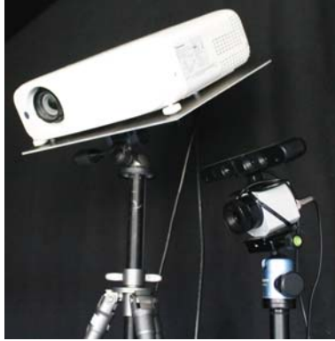
Fig. 3. Hardware used in the experiments, a Panasonic PT-VZ575N projector, an Asus Xtion Pro live RGB-D camera and an optris PI 400 thermal camera.
