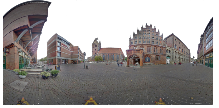
(b) Color panorama image with the Mercator projection built from a point cloud captured by Z+F IMAGER 5010C from city center of Hannover, Germany.
