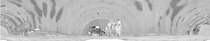
(c) Reflectance panorama image with equirectangular projection built from a point cloud captured by Riegl VZ-400 from inside a tunnel.
