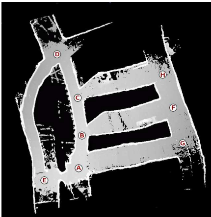
(a) Overview of the Kvarntorp data set. The robot travelled along the sequence A–B–C–D–E–A–F–G–A–B–C–H–F–H.
