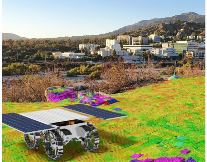
Fig. 1. CADRE rover with the CCM map. Image is generated by overlaying the super-sampled map (5 cm/cell map, sampled at 1 cm). The piece-wise linear map cells are visible as small inclined surfels with color indicating the variance normal to the slope and thus obstacle presence.
