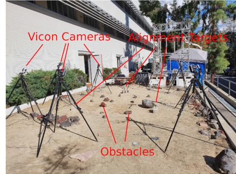
Fig. 8. Picture of the test setup at JPL.
