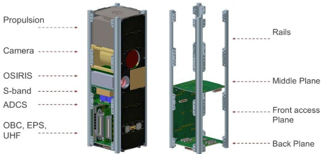
Fig.6 The set-up of each of the 3 TOM satellites with the structural components at the right, and the included subsystems and payloads at the left.
