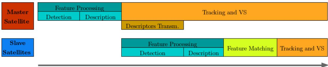
Fig. 5. Image processing pipeline for target tracking and image based visual servoing.
