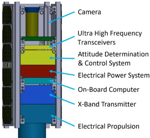
*Fig. 2. Typical small satellite design with camera payload in form of a 3Unit CubeSat (mass about 4 kg and dimension 30x10x10 cm)*
