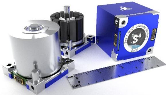
*Fig. 3. Miniature reaction wheel for satellite high precision pointing capabilities: in the background the brushless motor, at left the rotation mass on top of the motor, and at right the system finally sealed in its housing of a 2 cm cube.*
