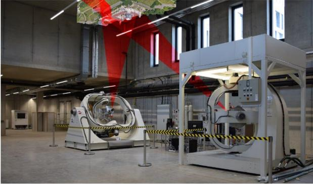
Fig. 8. Cameras mounted on the two precision turntables to simulate the orbit motion in imaging the 3D-object on the ceiling.
