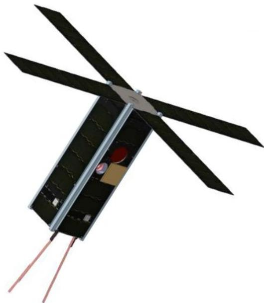
Fig. 7 TOM satellite with deployed solar arrays for power generation.
