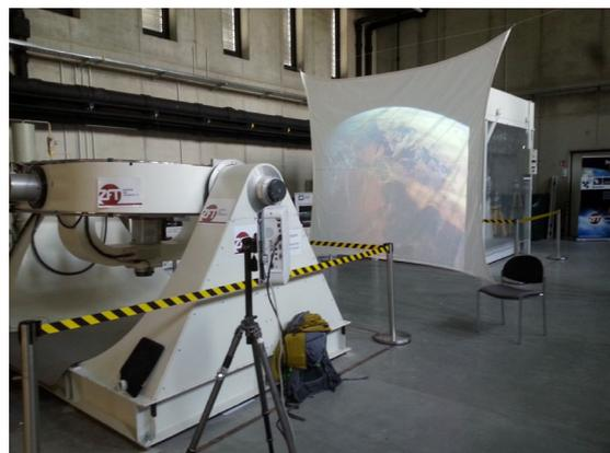
Fig. 8. Simulating Image Based Visual Servoing of a single satellite with a precision turntable.
