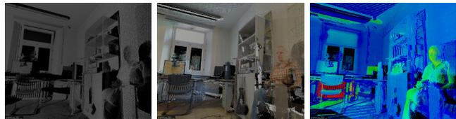
Fig. 1. Laser scan with reflectance, color and thermal information.
