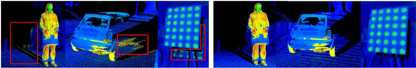
Fig. 2. Colored laser scan with errors (left) and with color correction (right).
