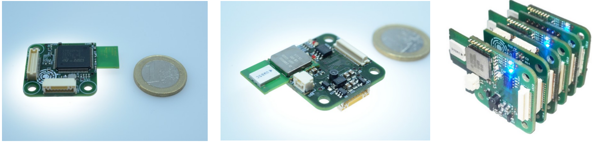
Figure 2: Left and middle: The SKITH-STM32 board, including the sticking out UWB-Tranceiver, comparing to a Euro coin. Right: Stacked SKITH-boards.
