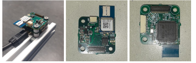
Fig. 4: The custom PCB with the UWB chip. Left: UWB PCB mounted in a stack with a USB communication board on the robot. Middle: The front of the PCB. Right: The back of the PCB.
