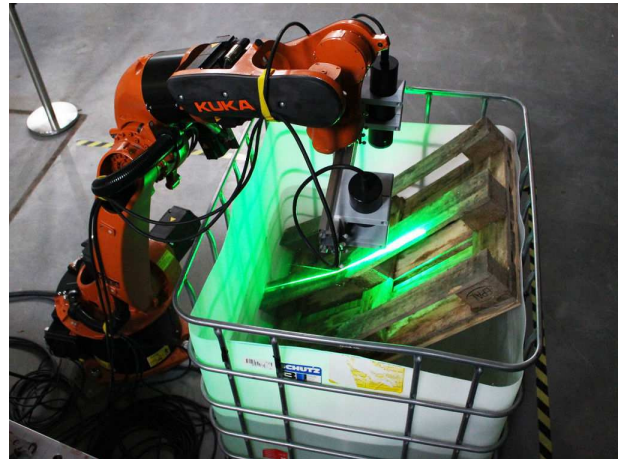
Figure 1. Prototype underwater line laser scanner mounted on an industrial manipulator for scanning a semi-submerged scene.
