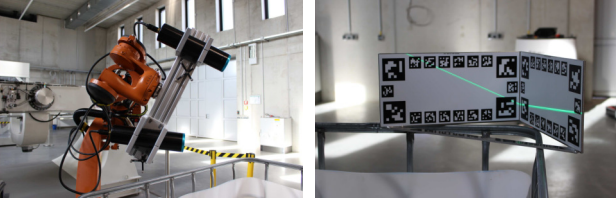
Figure 4. Calibration of the laser plane parameters using a L-shaped calibration target.
