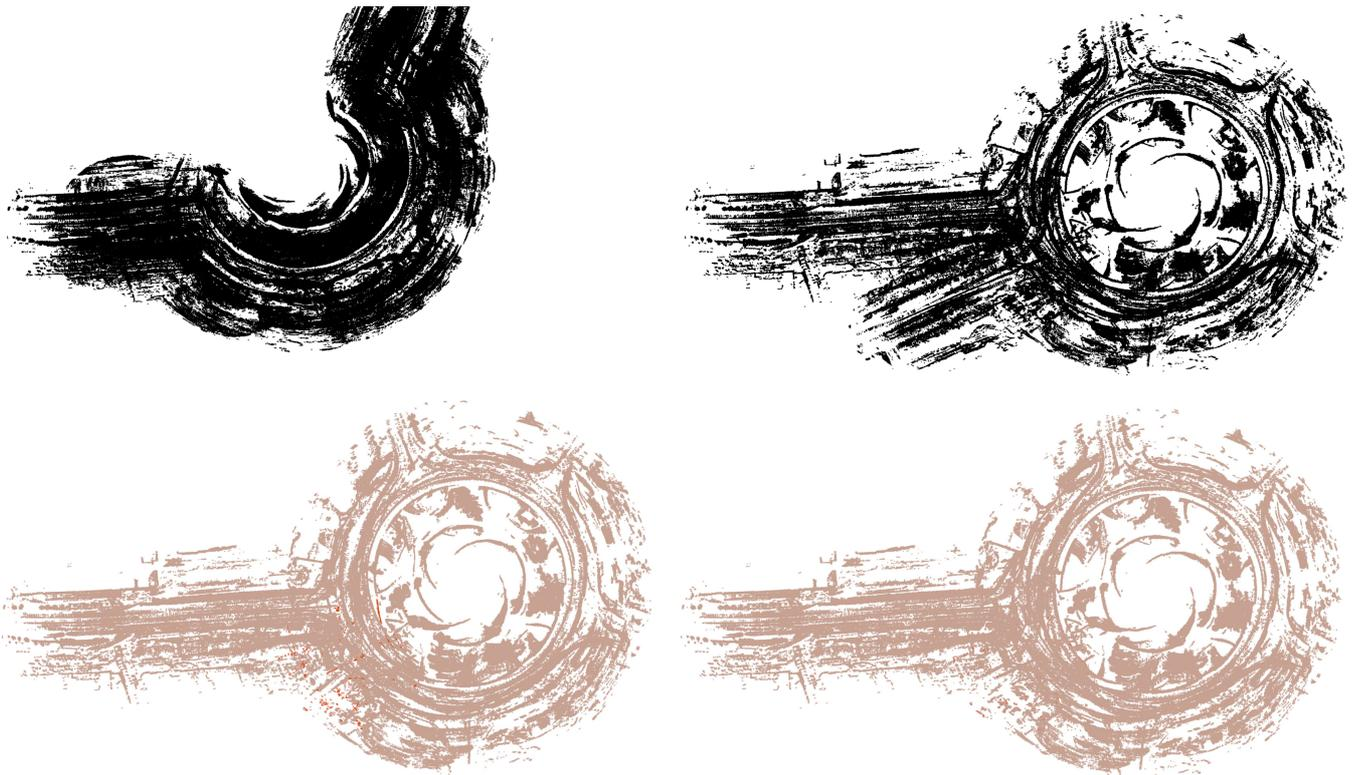
Figure 7. Mapping results using a Velodyne scanner. Top left: Plain vanilla ICP. Top right: Registration result using ICP and globally consistent scan matching. Bottom: ICP-based registration after removing ground points.
