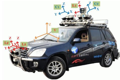
Figure 2. SmartV-II: An Autonomous car developed at Wuhan University.
