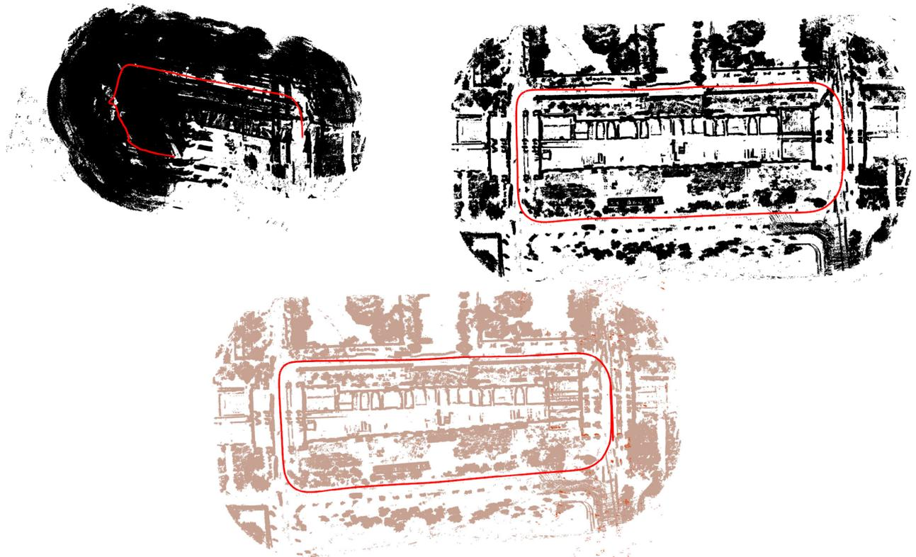
Figure 4. Mapping results using a Velodyne scanner. Top left: Plain vanilla ICP. Top right: Precise registration result using ICP and globally consistent scan matching. Bottom: ICP-based registration after removing ground points.
