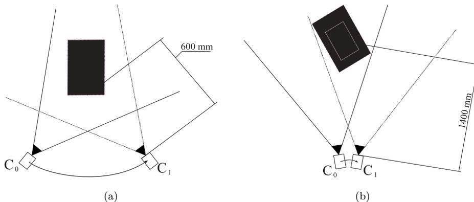
**Figure 13.** (a) Experimental setup *SI*: The camera was rotated by 90 deg around an object in a distance of 600 mm while it was kept centered in the field of view. The covered distance between  $C_0$  and  $C_1$  measured 950 mm. (b) Experimental setup *SII*: The camera was translated and rotated from  $C_0$  to  $C_1$  by 50 mm and 22 deg, respectively.
