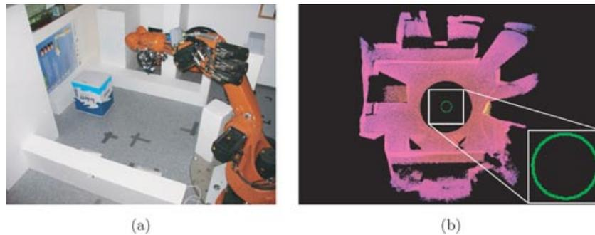
**Figure 14.** (a) Laboratory scene used for the ground truth evaluation. The ToF camera was mounted on an industrial robot arm (KUKA KR 16). (b) Bird's-eye view of the 3D map created by the use of provided robot poses (false color code relates distance to origin of coordinate system). The performed trajectory of circular shape is drawn at the lower right.
