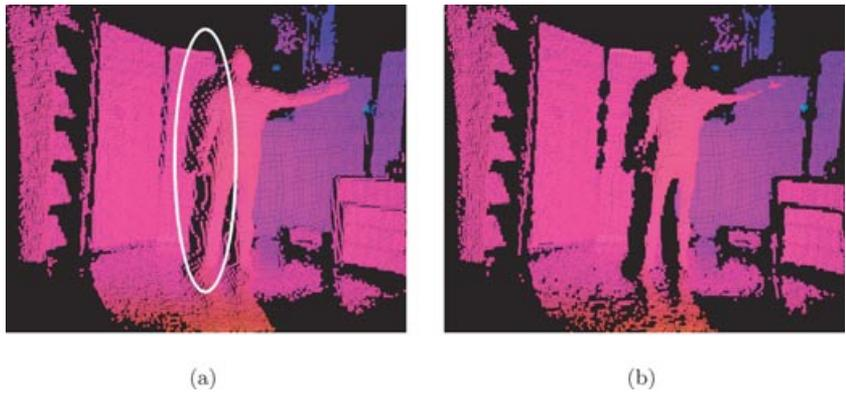
**Figure 4.** Jump edges occurring at the boundary of occluding shapes. (a) Unfiltered scene: A transition between the person in the foreground and the wall in the background can clearly be seen. (b) Filtered scene: Jump edges are reliably removed.
