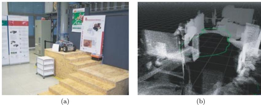
**Figure 31.** 3D mapping of a larger indoor environment—the robotics hall at Fraunhofer IAIS. (a) View of part of the hall. The environment contains different objects such as mobile filing cabinets, staircases, removable walls, and posters. (b) Perspective view of the registered 3D map of the hall. The performed trajectory (estimated poses of each frame) is drawn in green.
