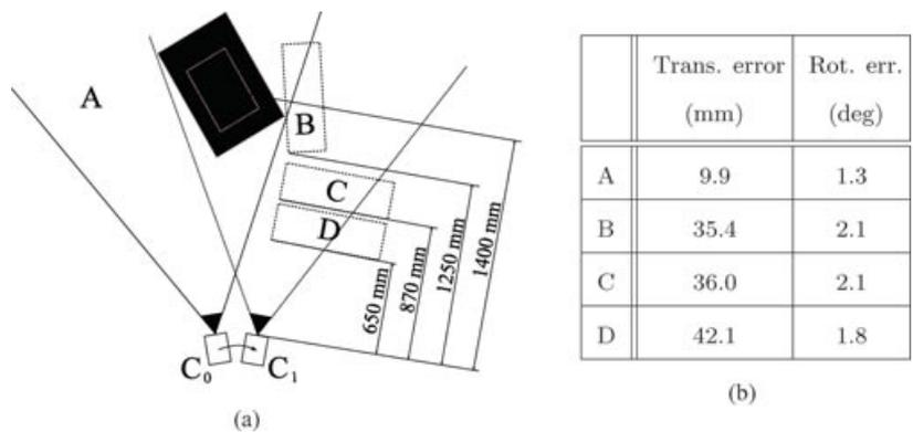
**Figure 18.** (a) Experimental setup for light-scattering investigations. The camera is moving from  $C_0$  to  $C_1$ . Initially, the scene consists of two Styrofoam cuboids standing on top of each other (case A). Then (cases B, C, and D), an additional Styrofoam cuboid was put into the scene. (b) Ego motion estimation results degrade from 9.9 to 42.1 mm due to light-scattering effects.
