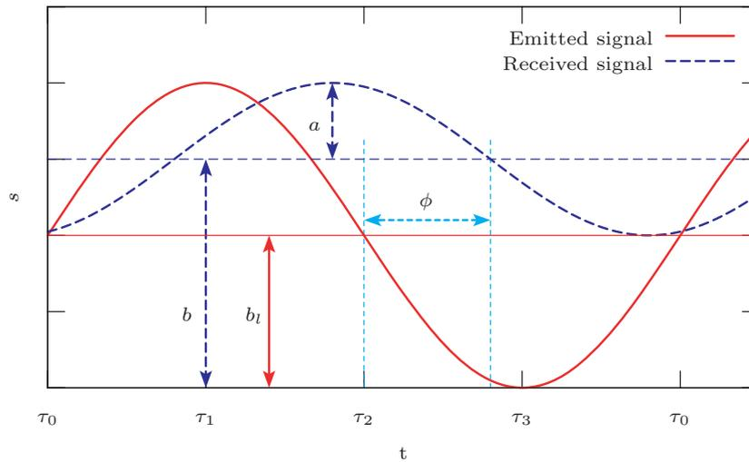
Figure 1. Received sinusoidally modulated input signal, sampled with four sampling points per modulation period  $T$ .
