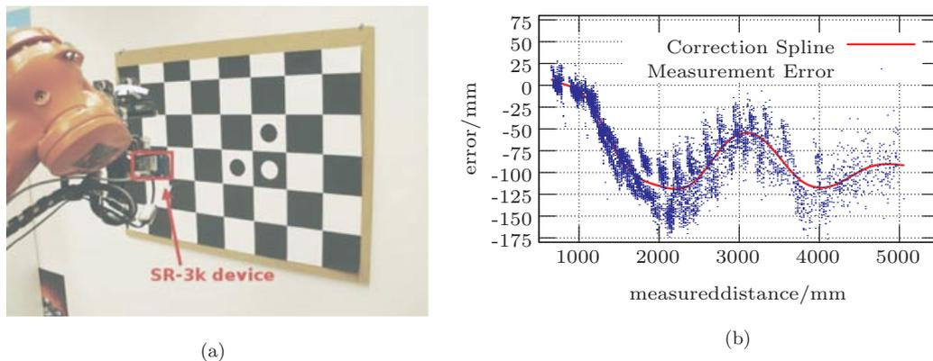
**Figure 7.** (a) The improved calibration is performed against a checkerboard pattern (image taken at the DLR laboratory). Pattern sizes  $1,190 \times 840$  mm. (b) The revealed depth measurement error varies from  $-150$  to  $10$  mm. For the most part the camera provides too-large-distance data. The spline approximates this error for subsequent correction purposes.
