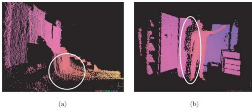
**Figure 2.** Interreflection effects due to multimodal reflections: (a) Corners or hollows appear rounded off. (b) Occluding shapes have a smooth transition.
