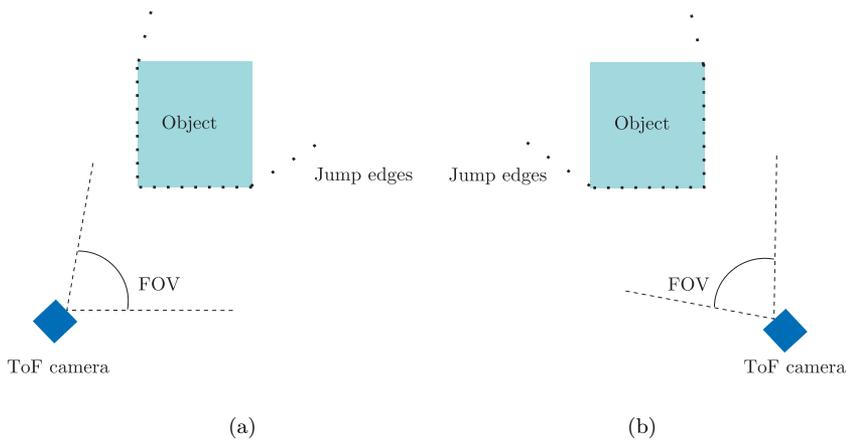
**Figure 5.** Jump edge appearance depends on the perspective view. The matching of both point clouds can easily result in a wrong registration.
