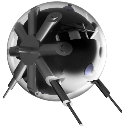
Figure 1. Rendering of the DAEDALUS robot concept. The spherical robot holds 2 rings with eight rods each on both sides. Apart from locomotion those rods are also used for tasks such as heat radiation, stabilization, and climbing. The main structure in the center holds laser scanners, optical sensors, a battery, a board computer and other payloads.
