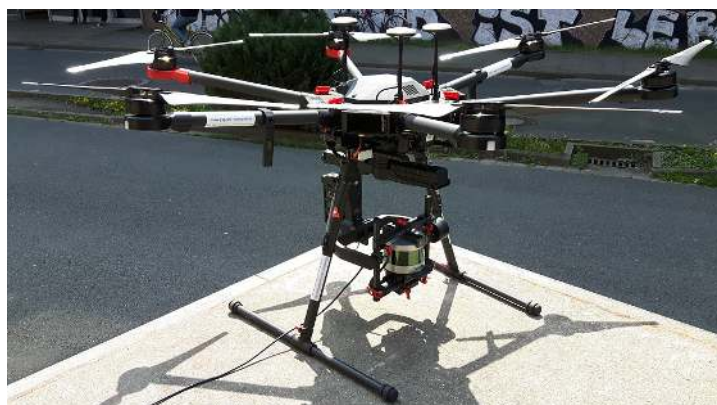
Figure 7. Overview of the prototype kinematic laser scanner-based UAV [53].
