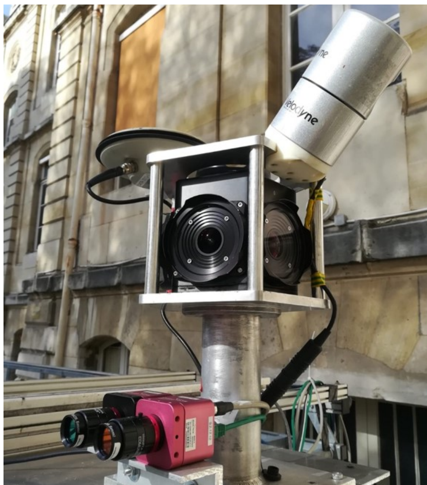
Figure 1. Prototype acquisition system used to create the PC3D dataset in the city of Paris. Sensors: Velodyne HDL32 LiDAR, Ladybug5 360^\circ camera, Photonfocus MV1 16-band VIR and 25-band NIR hyperspectral cameras (hyperspectral data are not available in this dataset; they cannot be used in mobile mapping due to the limited exposure time).
