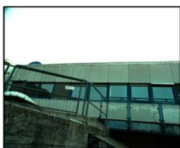
AE algorithm underexposed the surveyed object, negatively affected by the sky brightness
