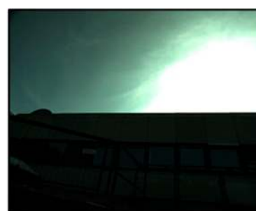
AE algorithm underexposed the surveyed object, negatively affected by the sky brightness
