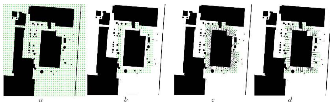
Figure 20. The initial sample viewpoints (a), the sample viewpoints located at the optimal range from the building (b), and the direction of each viewpoint for centre pointing (c) and façade pointing (d).
