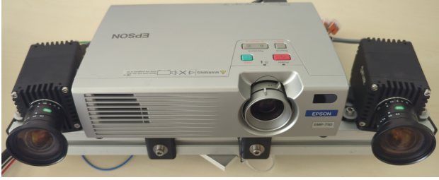
Figure 4. Experimental stereo camera system with mounted projector.
