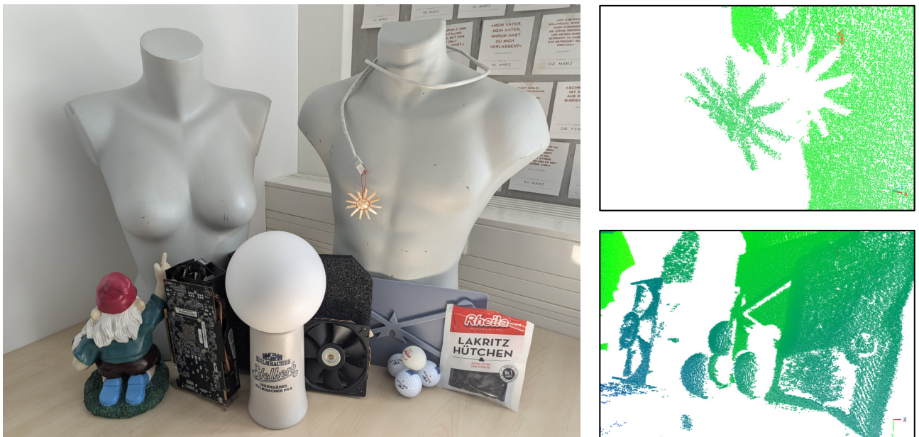
Figure 16. Reconstructed point clouds of the scene ‘Adam & Eve’, colored by depth. Top: Point cloud computed using 12 images with full descriptor generation. Black points are outliers present in the scan, which are missing when using limited descriptors and 33 images. Bottom left: overview of the scene. Bottom right: highlighted parts of the acquired point cloud, with both fine details of the ornament and accurate shapes of the PC fan, liquorice bag and golf balls. Other chosen parameters are: \theta_{NXC} = 0.96 , \theta_{Var} = 2.0 , \sigma_p = 0.1 .
