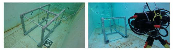
Figure 6. Scanning setup in the test tank. Left: Test structure constructed from aluminum profiles and polypropylene pipes, Right: Underwater laser scanner deployed on a tripod.
