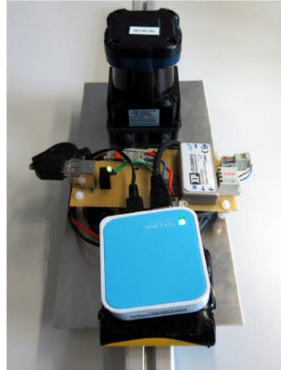
(b) Hardware setup of Hokuyo UTM-30LX-EW with independent power supply and wireless connection to run on the aisle.
