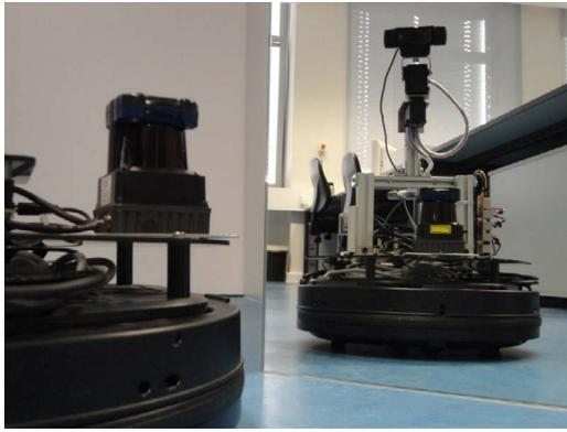
Fig. 1. Robot equipped with laser scanner facing an unframed mirror.
