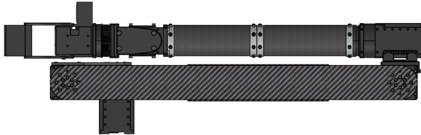
**Figure 3.** CAD drawing of the initial pose of the robot arm,  $\varphi_1 \dots \varphi_6 = 0$  rad.
