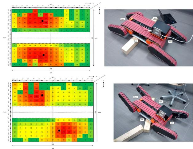
Fig. 4. Sensor feedback and pressure distribution for predictive mobility, safe and stable execution during manipulation tasks
