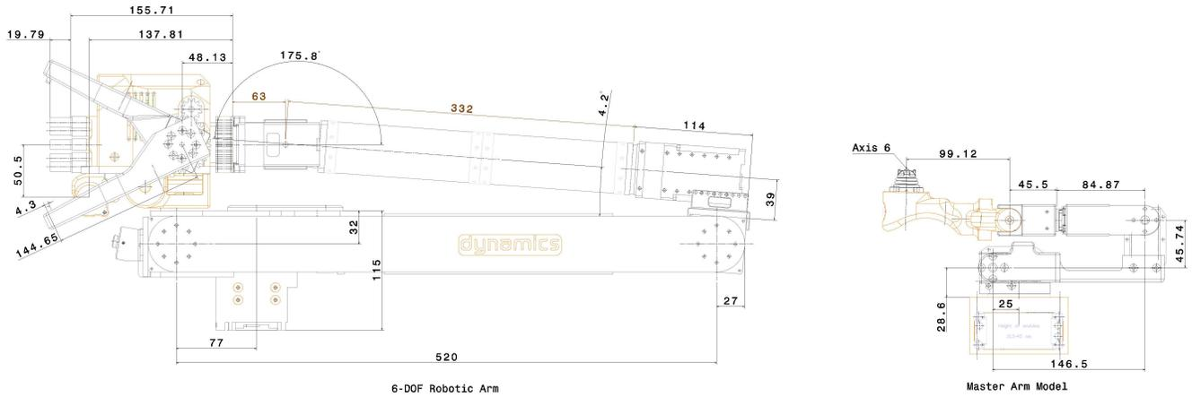
Fig. 3. Configuration, link lengths and coordinates mapping of the small-size 6-DOF robotic manipulator and the corresponding master arm controller.
