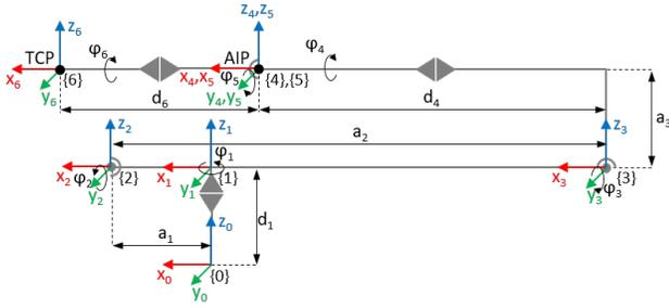
Fig. 5. Schematic sketch of the robot arm with assigned coordinate systems used for forward and inverse kinematics,  $\varphi_1 \dots \varphi_6 = 0 \text{ rad}$
