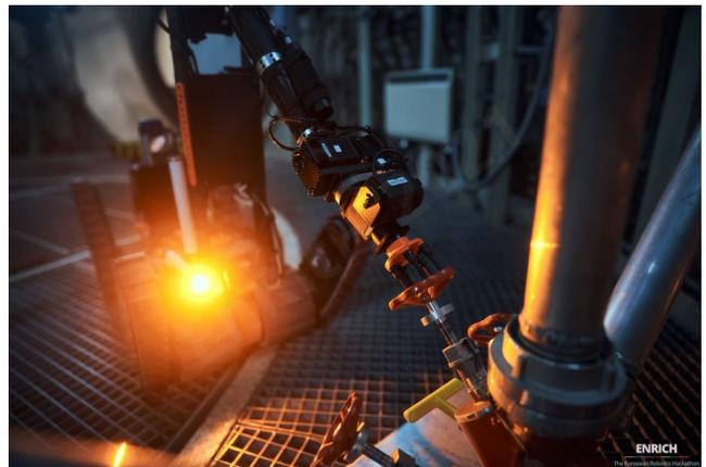
Fig. 7. Valve closing at EnRiCh in NPP Zwentendorf
