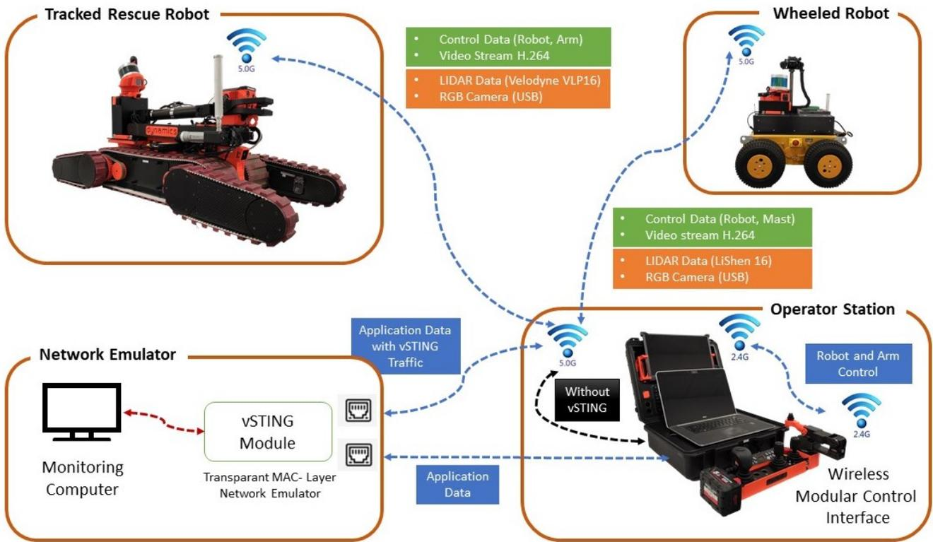
Fig. 6. Cross-domain application of the STING (Spatially Distributed Traffic and Incident Generation) concept from TU Dortmund [26] for testing the resilience of mission-critical human-robot communications.
