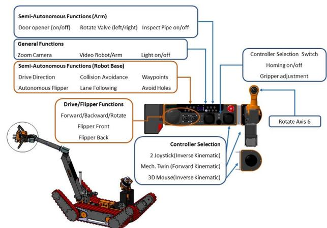
Fig. 2. HRI overview: A tracked rescue robotic system with a 6-DOF manipulator and multi-functional gripping system (left) and a modular User-Interface for controlling the mobile system with a master arm controller/3D mouse controller
