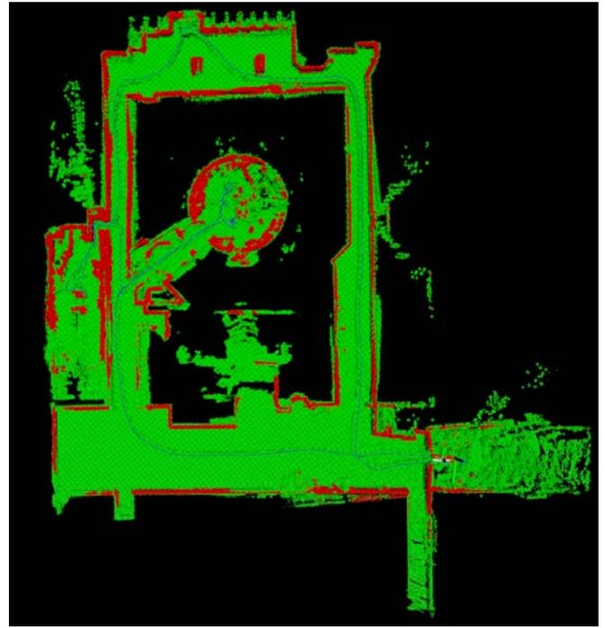
Fig. 6. Top view of 3D traversability model of an NPP and robot path (blue line): Traversability terrain prediction as green grid cells and Non-Traversability marked as red cells;
