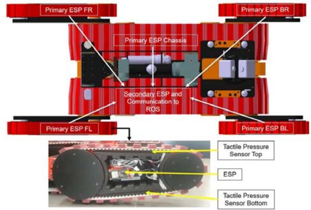
Fig. 4. ESP-based sensor communication setup: Each sensor module (primary) in the flipper system has been equipped with its own power supply due to the design of the robot and thus acts as a standalone unit. The rotational movement of the flippers can be adjusted from 0-360°, which means that support for a tactile sensor is installed at the top as well as at the bottom side.
