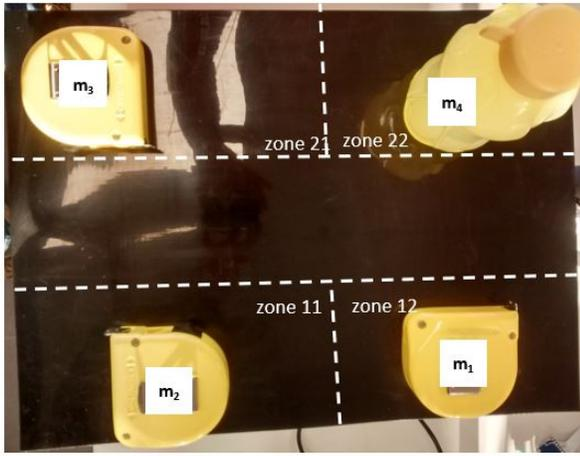
Fig. 5. Principle measurement setup with different objects with the flipped pressure distribution.
