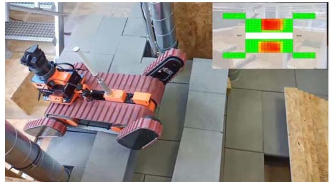
Fig. 7. HRI: Visualization of the tactile sensor data and visual feedback for the operator.
