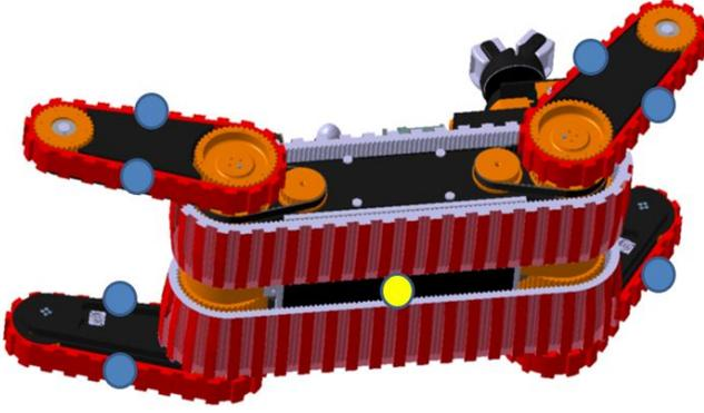
Fig. 3. Sensor Concept for Terrain Feedback: Yellow marker indicates sensitive pressure sensor for center tracks, while blue indicates in sum eight pressure sensor units for the flipper system. Due to the mechanical construction, either the front or the rear flipper system can be rotated inwards.
