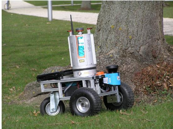
**Fig. 1.** The mobile robot Irma3D (Intelligent robot for mapping applications in 3D) with its main sensor, the RIEGL VZ-400.
