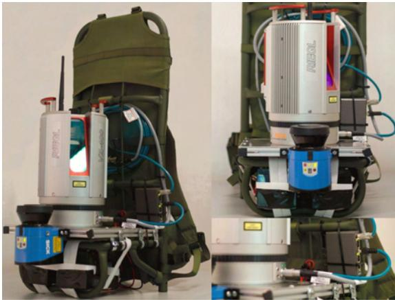
Figure 6: Images of the backpack system. Left: Side view with all of its sensors and equipment. Right: Detailed view of the SICK and the switch.
