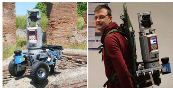
Figure 1: Left: The robot Irma3D. Videos of the system are available at <http://www.youtube.com/AutomationAtJacobs> Right: The backpack mobile mapping system.
