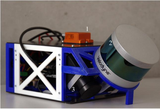
Fig. 1: The sensor unit featuring a Xsens Mti-G 700 (1) IMU, a Velodyne VLP16 Lite (2) laser scanner and an Optris PI 640 LW (3) thermal camera.
