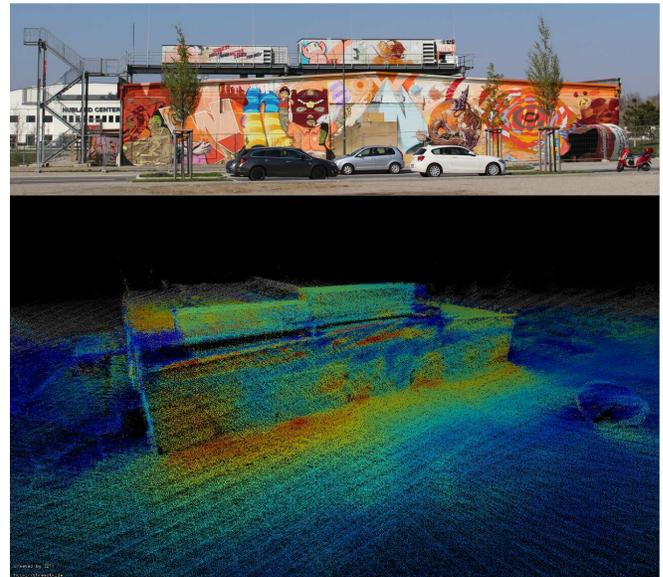
Fig. 7: The Food Court, Würzburg a former mall. The building is covered with graffiti (above), also apparent in the point cloud colored by temperature (below). Red color indicates higher temperatures, blue color lower temperatures
