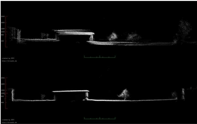
Fig. 6: Cross section of the initial (above) and the optimized point cloud (below)
