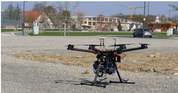
Fig. 4: Multicopter equipped with the sensor payload at the landing field during a test mission.
