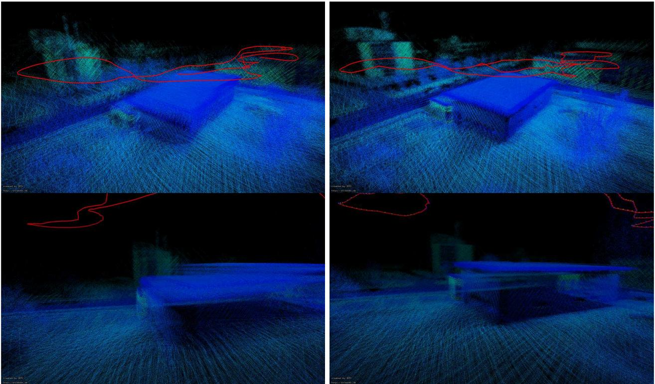
Fig. 5: Point cloud of the robotics hall from two perspectives with initial pose estimation (left) and after applying continuous-time ICP (right). The point clouds are colored by reflectance values. The red line resembles the trajectory.
