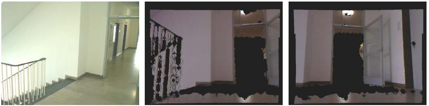
Fig. 2. Scene 1 for evaluation: Left) Scene in line of sight during rotational movement. Center/Right) Two range images with low overlap were taken. Depicted is the perspective view of the Kinect device. It can be noticed that specular reflections avoid distance measurements when the emitted light hits the ground under an obtuse angle. Black areas were either not in line of sight or incapable of measurement due to reflections or external lighting.
