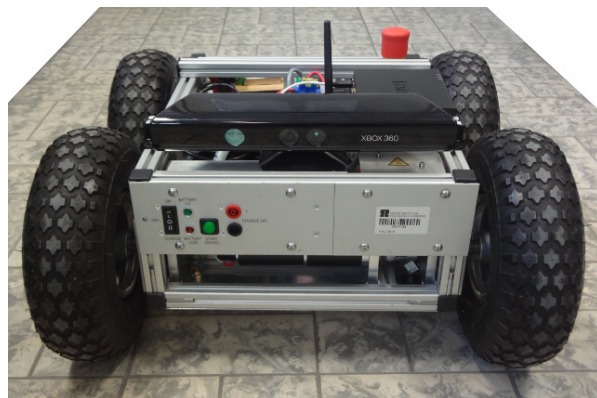
Fig. 1. Robot equipped with a Kinect device for 3D mapping purposes in indoor environments.
