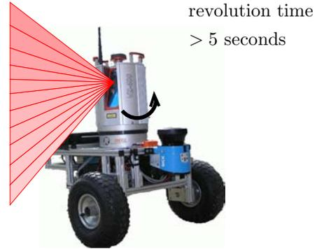
Fig. 1. The mobile robot Irma3D with its sensor: RIEGL VZ400, SICK LMS100, xsens gyro and wheel encoders. The VZ400 needs at least 6 seconds for one revolution.
