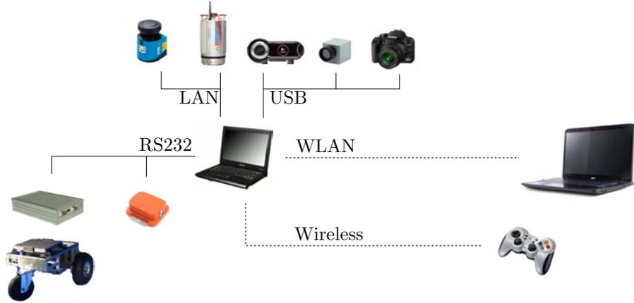
Fig. 2. System network. Components are connected by RS232, USB and LAN. Control is provided by a wireless joystick or a base station running an user interface.
